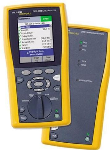
Figura 7 - DTX Cable Analyzer
